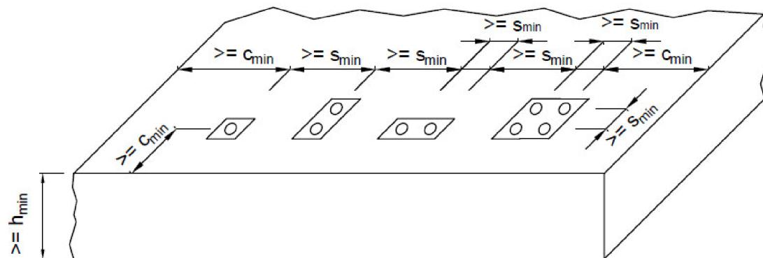
The spacing, edge distances and min. thicknesses of concrete member apply analogously when installing sockets in the end face of concrete member.
