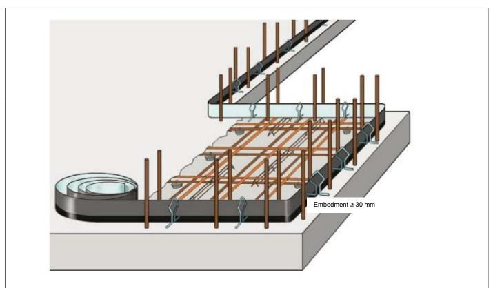
Coated metal water stop "Dichtblech VB" - single or double coated - for construction joints
