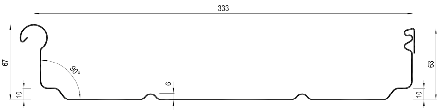
RIB-ROOF Evolution cover width = 333 mm
