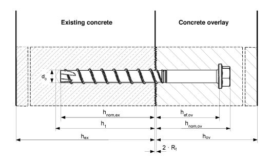
h<sub>nom,ex</sub> Overall embedment depth in existing concrete
