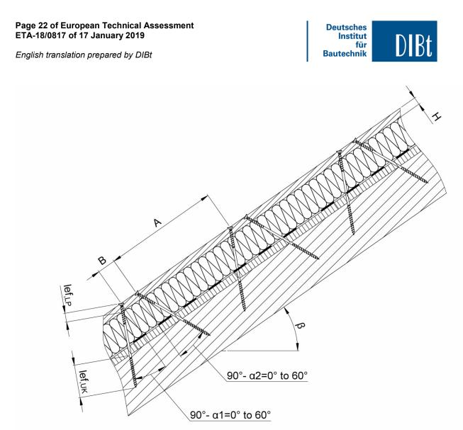
Figure A.4.4 Fastening of thermal insulation material on top of rafters - structural system for alternatively inclined screws
