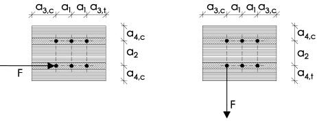
Figure A.2.2 Definition of spacing, end and edge distances in the edge surface of the cross laminated timber. For screws in the edge surface,  $a_1$  and  $a_3$  are parallel to the CLT plane face,  $a_2$  and  $a_4$  perpendicular to CLT plane face.
