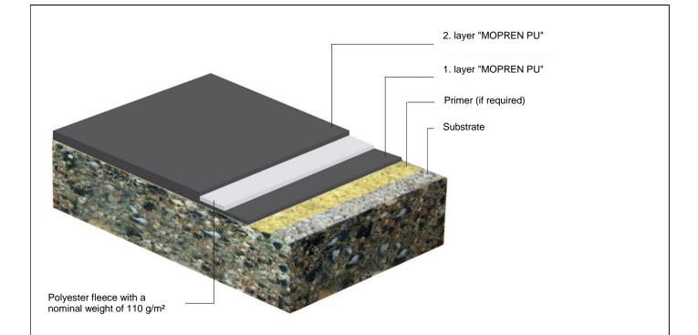
Applicable to the roof waterproofing "MOPREN PU"
