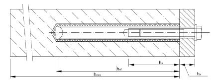
$t_{\text{fix}}$  = thickness of fixture
