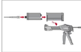
Tightly attach Hilti mixing nozzle HIT-RE-M to foil pack manifold. Do not modify the mixing nozzle.
