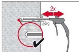
Blow 2 times from the back of the hole over the whole length with oil-free compressed air (min. 6 bar at 6 m<sup>3</sup>/h) until return air stream is free of noticeable dust.
