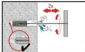
Brush 2 times with the specified brush (see Table B3) by inserting the steel brush Hilti HIT-RB to the back of the hole in a twisting motion and removing it.
