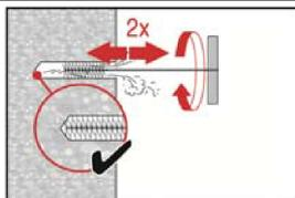
Brush 2 times with the specified brush (see Table B3) by inserting the steel brush Hilti HIT-RB to the back of the hole in a twisting motion and removing it.
