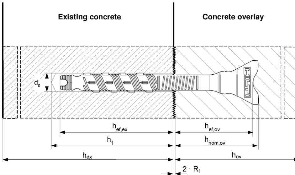
$h_{ef,ex}$  Effective embedment depth in existing concrete
