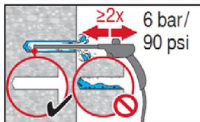
Blow 2 times from the back of the hole over the whole length with oil-free compressed air (min. 6 bar at 6 m<sup>3</sup>/h) until return air stream is free of noticeable dust and water.
