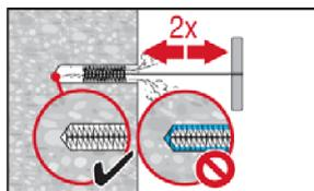
Brush 2 times with the specified brush size (brush  $\varnothing \geq$  drill hole  $\varnothing$ , see Table B3) by inserting the steel brush Hilti HIT-RB to the back of the hole in a twisting motion and removing it.
