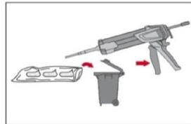
The foil pack opens automatically as dispensing is initiated. Depending on the size of the foil pack an initial amount of adhesive has to be discarded. Discarded quantities are:
