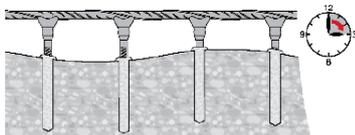
Observe the curing time  $t_{cure}$ , which varies according to temperature of base material (see Table B4). After  $t_{cure}$  has elapsed the concrete overlay can be concreted.
