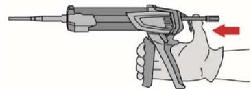
After injection is completed, depressurize the dispenser by pressing the release trigger. This will prevent further adhesive discharge from the mixer.
