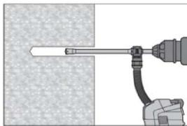
Drill hole to the required embedment depth with an appropriately sized Hilti TE-CD or TE-YD hollow drill bit attached to Hilti vacuum cleaner VC 20/40 (-Y) (suction volume  $\geq 57$  l/s) with automatic cleaning of the filter activated. This drilling system removes the dust and cleans the drill hole during drilling when used in accordance with the user's manual. After drilling is completed, proceed to the "injection preparation" step in the installation instruction.
