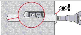
After injection is completed the annular gap must be completely filled with mortar. Excess mortar flows out of the borehole.
