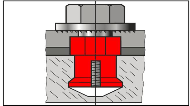
b) Installed anchor
