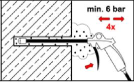
Finally blow the hole clean again with compressed air (min. 6 bar) **four** times. If the bore hole ground is not reached an extension shall be used.
