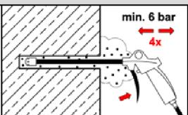
Starting from the bottom or back of the bore hole, blow out the hole with compressed air (min. 6 bar) **four** times.
