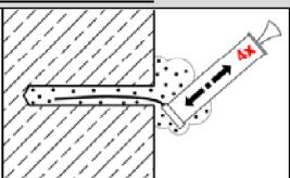
Starting from the bottom or back of the bore hole, blow the hole clean with the blow-out pump **four** times.
