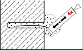
Finally blow the hole clean again with the blow-out pump **four** times.
