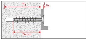
Countersunk Head : SK-CS 10B21 (SK8, SK10) A4 (SK8, SK10)
