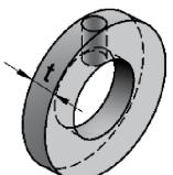
Thickness of washer with bore
