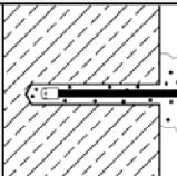
Starting from the bottom or back of the bore hole, blow out the hole with compressed air (min. 6 bar) a minimum of <b>two</b> times until return air stream is free of noticeable dust.<br>If the borehole ground is not reached, an extension must be used.                                                                                 |  |  |  |
