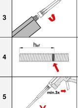
Attach the supplied static-mixing nozzle to the cartridge and load the cartridge into the correct dispensing tool.
