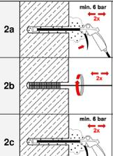
Starting from the bottom or back of the bore hole, blow out the hole with compressed air (min. 6 bar) a minimum of **two** times until return air stream is free of noticeable dust.
