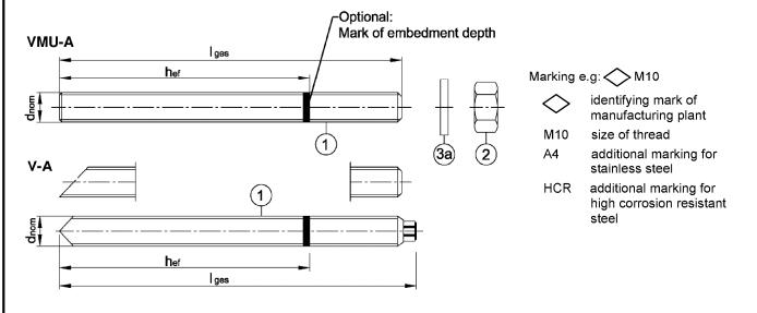
Threaded rod VM-A (material sold by the meter, to be cut at the required length) M8, M10, M12, M16, M20, M24, M27, M30 (zinc plated, A2, A4, HCR)
