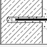
Starting from the bottom or back of the bore hole, blow out the hole with compressed air (min. 6 bar) again a minimum of <b>two</b> times until return air stream is free of noticeable dust.<br>If the borehole ground is not reached, an extension must be used.                                                                         |  |  |  |
