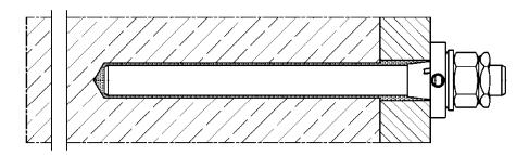
fischer anchor rod RG M with fischer mortar capsule system RSB
