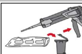
The foil pack opens automatically as dispensing is initiated. Depending on the size of the foil pack, an initial amount of adhesive has to be discarded. Discarded quantities are
