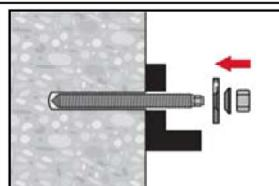
Use Hilti Filling Set with standard nut. Observe the correct orientation of filling washer and spherical washer.
