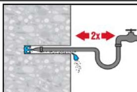
Flush 2 times by inserting a water hose (water-line pressure) to the back of the hole until water runs clear.
