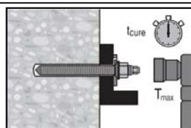
The applied installation torque shall not exceed the values  $T_{max}$  given in Table B2 to Table B5.
