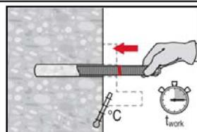
Before use, verify that the element is dry and free of oil and other contaminants. Mark and set element to the required embedment depth before working time  $t_{work}$  has elapsed. The working time  $t_{work}$  is given in Table B7.
