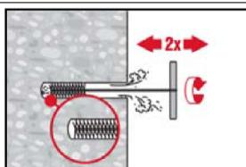
Brush 2 times with the specified brush (see Table B8) by inserting the steel brush Hilti HIT-RB to the back of the hole (if needed with extension) in a twisting motion and removing it. The brush must produce natural resistance as it enters the drill hole (brush  $\varnothing \geq$  drill hole  $\varnothing$ ) - if not the brush is too small and must be replaced with the proper brush diameter.
