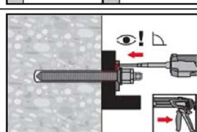
Fill the annular gap between anchor rod and fixture with 1-3 strokes of a Hilti injection mortar HIT-HY ... or HIT-RE ... .
