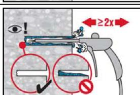
Blow 2 times from the back of the hole (if needed with nozzle extension) over the whole length with oil-free compressed air (min. 6 bar at 6 m<sup>3</sup>/h) until return air stream is free of noticeable dust and water. Remove all water from the drillhole until drillhole is completely dried before mortar injection. For drill hole diameters  $\geq 32$  mm the compressor has to supply a minimum air flow of 140 m<sup>3</sup>/h.
