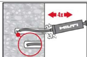
The Hilti hand pump may be used for blowing out drill holes up to diameters  $d_0 \leq 20 \text{ mm}$  and drill hole depths  $h_0 \leq 10 \cdot d$ .
