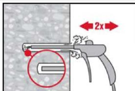
Blow 2 times from the back of the hole (if needed with nozzle extension) over the hole length with oil-free compressed air (min. 6 bar at 6 m<sup>3</sup>/h) until return air stream is free of noticeable dust.
