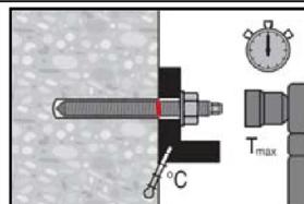
Loading the anchor: After required curing time  $t_{cure}$  (see Table B7) the anchor can be loaded.
