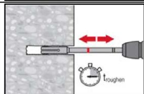
Before roughening water needs to be removed from the drill hole. Check usability of the roughening tool with the wear gauge RTG. Roughen the drill hole over the whole length to the required  $h_{\text{ref}}$ .
