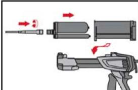
Tightly attach Hilti mixing nozzle HIT-RE-M to foil pack manifold. Do not modify the mixing nozzle.
