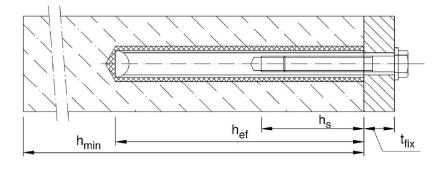
$t_{fix}$  = thickness of fixture
