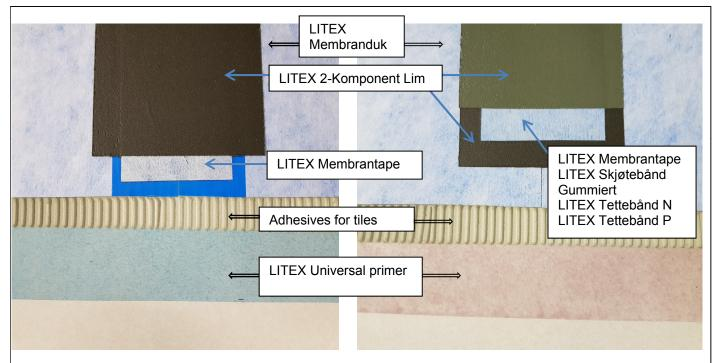
Minimum layer thickness of the waterproofing sheet 0.6 mm
