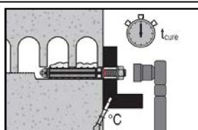
After required curing time  $t_{cure}$  (see Table B9 and Table B10) the anchor can be loaded.
