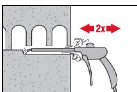
Blow again with Hilti hand pump or compressed air 2 times until return air stream is free of noticeable dust.
