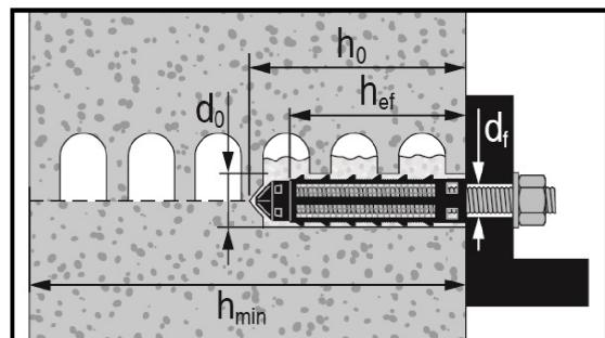
**Figure A2:** Hollow and solid brick with HAS-U-... and two sieve sleeves HIT-SC for deeper embedment depth (see Table B6)
