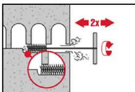
Brush 2 times with the specified steel brush (tables B5 to B8) by inserting the steel brush Hilti HIT-RB to the back of the hole (if needed with extension) in a twisting motion and removing it.
