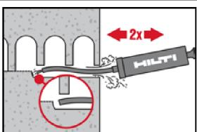
The Hilti hand pump may be used for blowing out drill holes up to diameters  $d_0 \leq 18$  mm and drill hole depths up to  $h_0 = 100$  mm.
