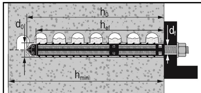
**Figure A3:** Solid brick with HAS-U-... (see Table B7)
