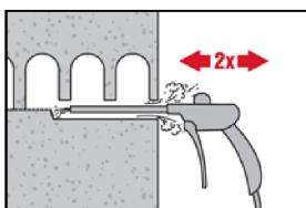
Blow 2 times from the back of the hole (if needed with nozzle extension) over the hole length with oil-free compressed air (min. 6 bar at 6 m<sup>3</sup>/h; drill hole depth up to  $h_0 = 300$  mm) until return air stream is free of noticeable dust.
