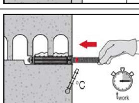
Set element to the required embedment depth until working time  $t_{work}$  has elapsed. The working time  $t_{work}$  is given in Table B9 and Table B10.
