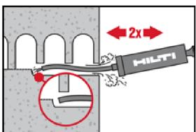
Blow out again with the Hilti hand pump at least 2 times until return air stream is free of noticeable dust.
