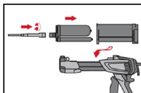
Tightly attach new Hilti mixing nozzle HIT-RE-M to foil pack manifold (snug fit).
