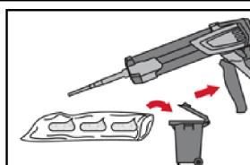
Discard initial adhesive. The foil pack opens automatically as dispensing is
