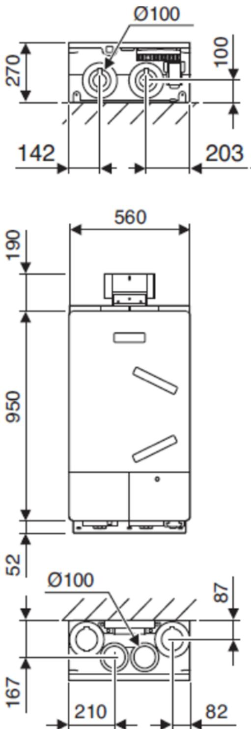
Abmessungen in [mm]
