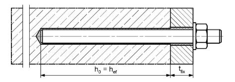
Pre-positioned or push through installation with subsequently injected filling disk (annular gap filled with mortar)
