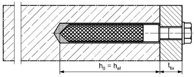
Pre-positioned installation with subsequently injected filling disk (annular gap filled with mortar)
