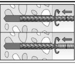
Only use clean and oil-free reinforcing bars or fischer FRA. Mark the setting depth. Turn while using force to push the reinforcement bar or the fischer FRA into the filled hole up to the setting depth mark
