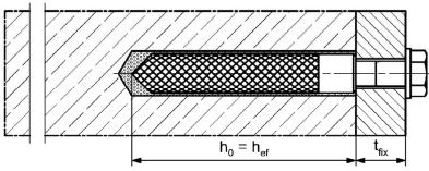
Pre-positioned installation with subsequently injected BERNER filling disc (annular gap filled with mortar)
