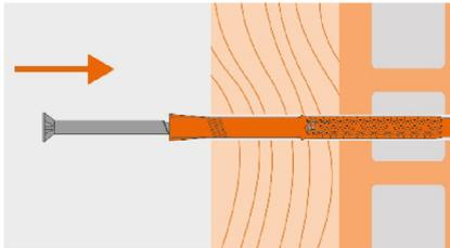
Setting the anchor with the preassembled fastener through the part to be fixed.
