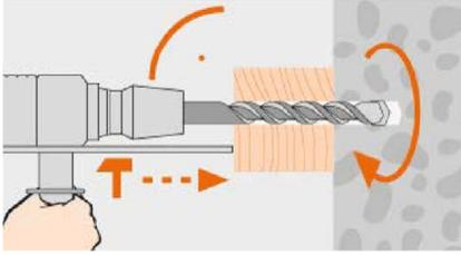
Drill the hole by **hammer drilling**.
