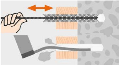
Pre-cleaning the drill hole with a brush, then hole-blowing with a pump.
