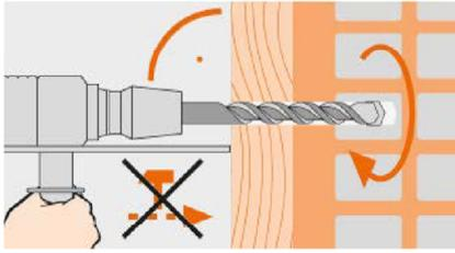
Drill the hole according to the method given in Table C6 and C7 by **rotary drilling** (without hammering) or **hammer drilling**.
