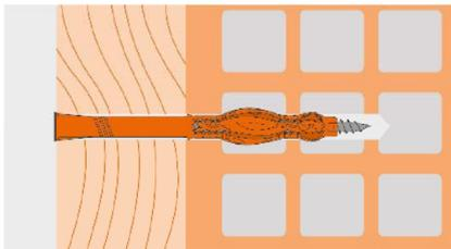
Tighten the fastener until sleeve collar contact.
