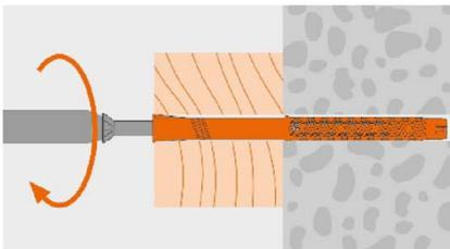
Push the anchor till the collar of the sleeve contacts the part to be fixed, then fix the part with screw.
