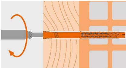
Push the anchor until the collar contacts the part to be fixed, then fix the part with screw.
