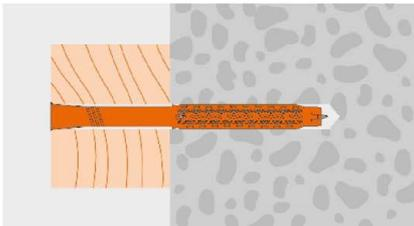
Tightening the fastener until sleeve collar contact.
