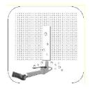
Blow out dust from drilling hole.
