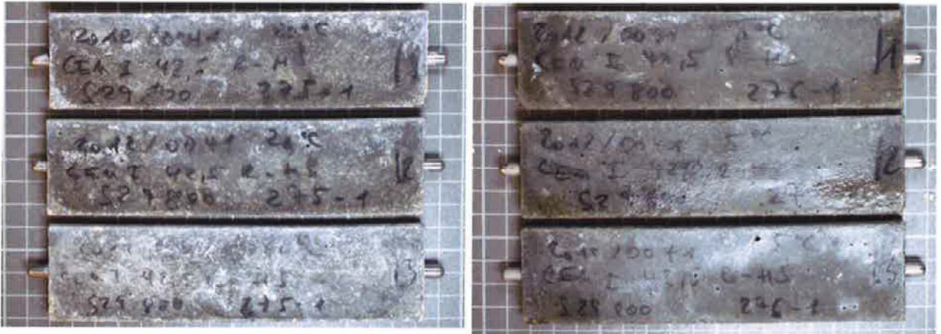
Figures A5: Flat prism from Portland cement CEM I 42,5 R-SR0 after 180 days storage in \text{Na}_2\text{SO}_4 -solutions at 20 °C (on the left) and 5 °C (on the right)
