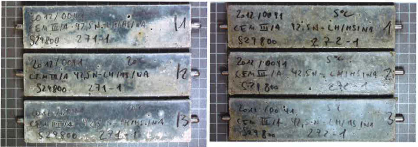
Figure A3: Flat prism from blast furnace cement CEM III/A 42,5 N-LH/SR/LA "Deuna" (C2) with blast furnace 2 (S2) after 180 days storage in Na 2 SO 4 -solutions at 20 °C (on the left) and 5 °C (on the right)
