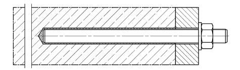
Push through installation (annular gap filled with mortar)
