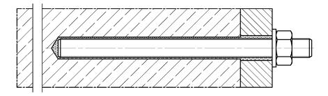
Pre-positioned or push through installation with subsequently injected fischer filling disc (annular gap filled with mortar)
