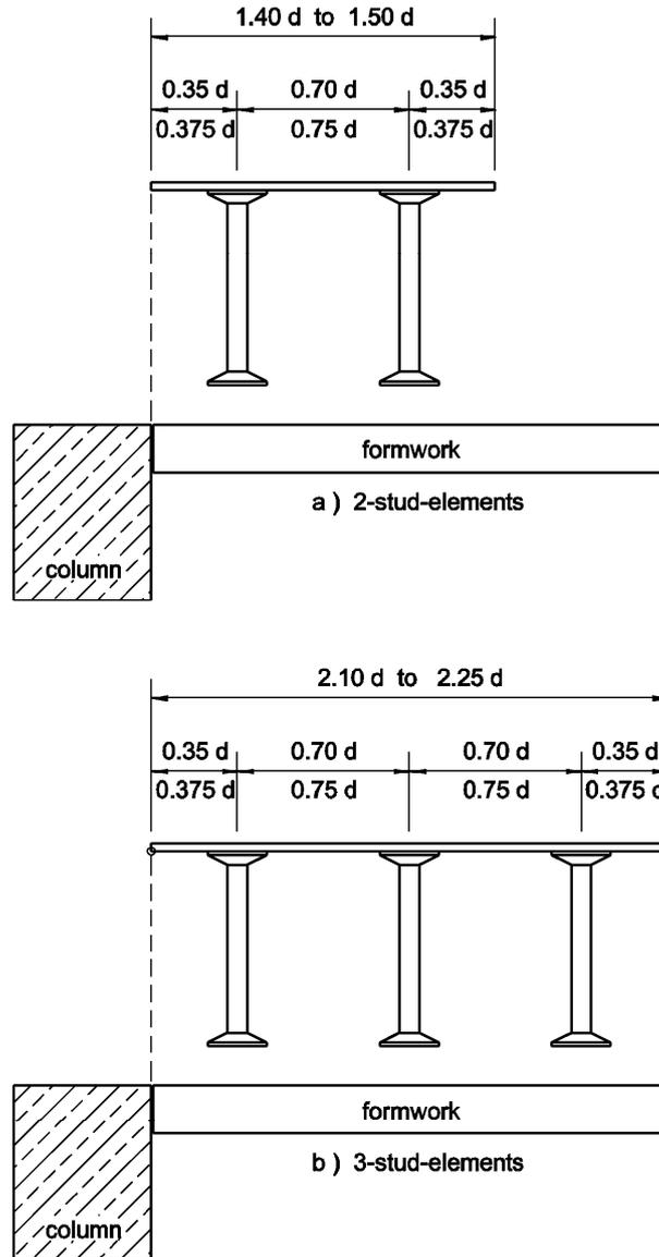
HALFEN HDB double headed studs for punching shear reinforcements
