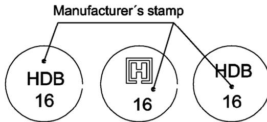
Material: reinforcement steel with a characteristic yield strength of  $f_{yk} \geq 500$  MPa acc. to EN 1992-1-1, annex C and provided data sheet
