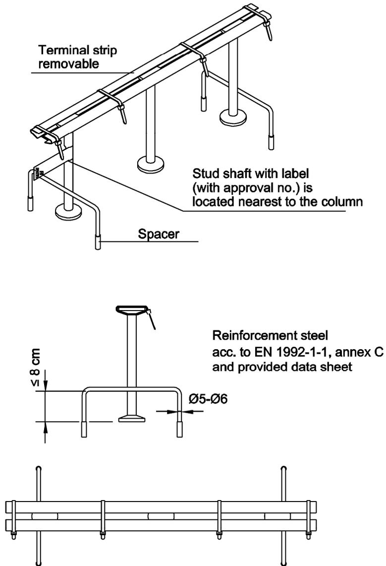
HALFEN HDB double headed studs for punching shear reinforcements
