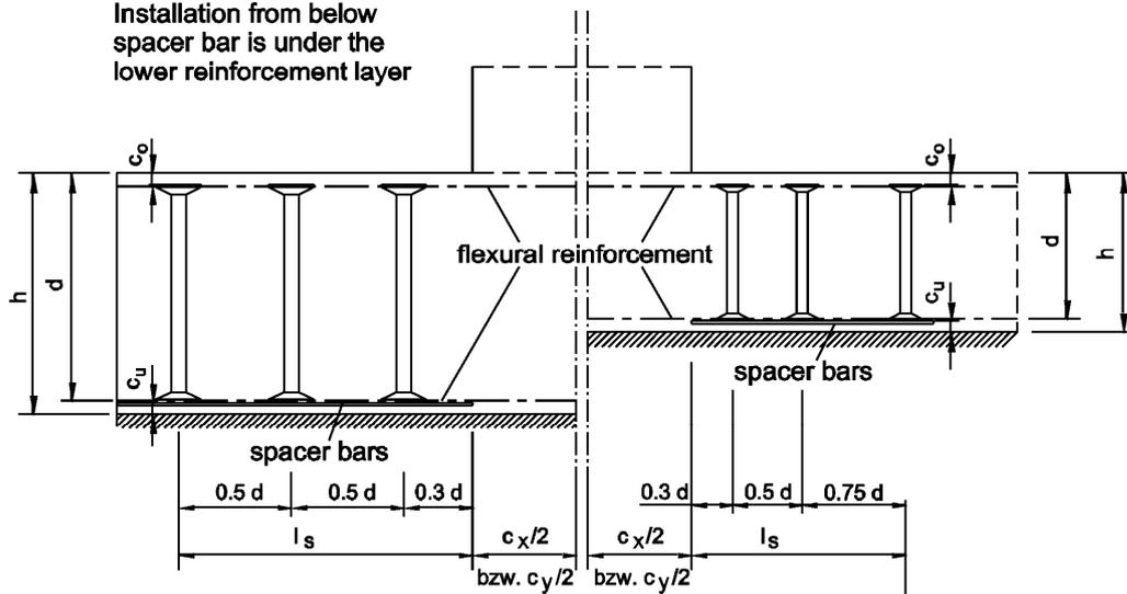
Concrete cover  $c_o$  resp.  $c_u$  acc. to EN1992-1-1 : 2004 + AC : 2010, section 4.4
