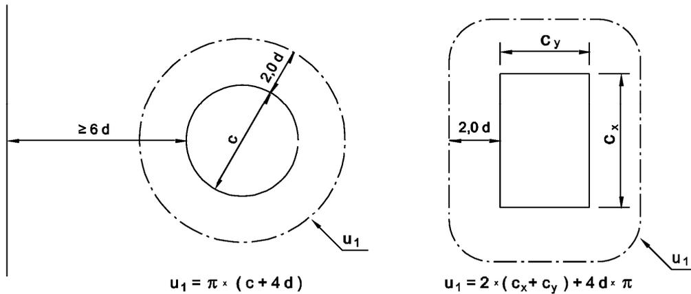
b) Loaded areas (columns) are less than  $6d$  from openings (voids) in the slab.
