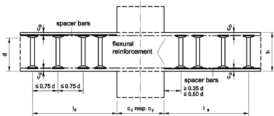
Concrete cover  $c_o$  resp.  $c_u$  acc. to EN1992-1-1 : 2004 + AC : 2010, section 4.4
