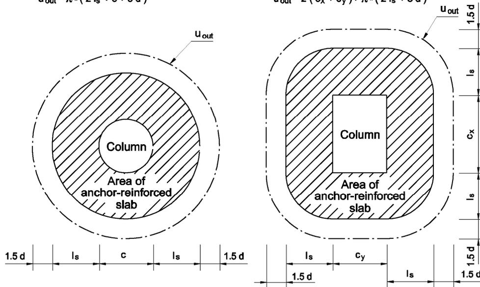
HALFEN HDB double headed studs for punching shear reinforcement
