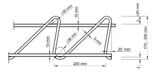
Material: reinforcement steel according EN 1992-1-1, Annex C with a characteristic yield strength of  $f_{yk} = 500 \text{ N/mm}^2$
