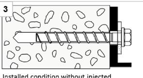
Installed condition without injected mortar in the filling washer
