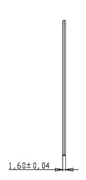
Staple raw wire: ø 1,53±0,03mm Tensile strength  $\geq$  900 N/mm<sup>2</sup> round stainless steel wire WNr. 1.4301 / 1.4401 / 1.4529 or galvanised round wire with zinc thickness  $\geq$  86 g/m<sup>2</sup> Resin coating  $L_H = min. 0.5 L_n$ ;  $\geq 20mm$  Leg length  $L_n = 25.0 - 100.0mm$
