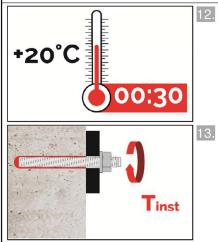
After full curing, the add-on part can be installed with up to the max. torque (Table B1 or B3) by using a calibrated torque wrench. In case of prepositioned installation the annular gab between anchor and fixture can be optional filled with mortar. Therefor substitute the washer by the filling washer and connect the mixer reduction nozzle to the tip of the mixer. The annular gap is filled with mortar,
