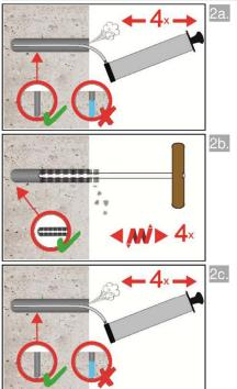
Starting from the bottom or back of the bore hole, blow the hole clean with handpump (Annex B 4) a minimum of four times until return air stream is free of noticeable dust.
