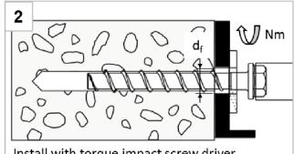
Install with torque impact screw driver or torque wrench
