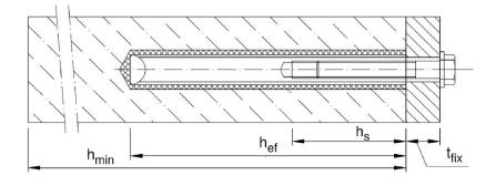
$t_{fix}$  = thickness of fixture
