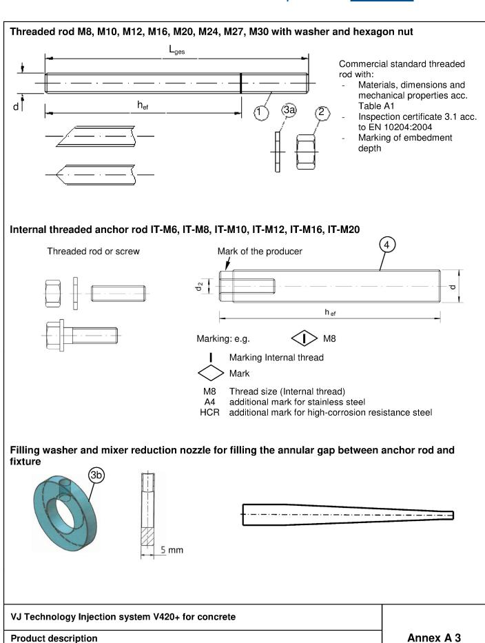
Threaded rod, internal threaded rod and filling washer
