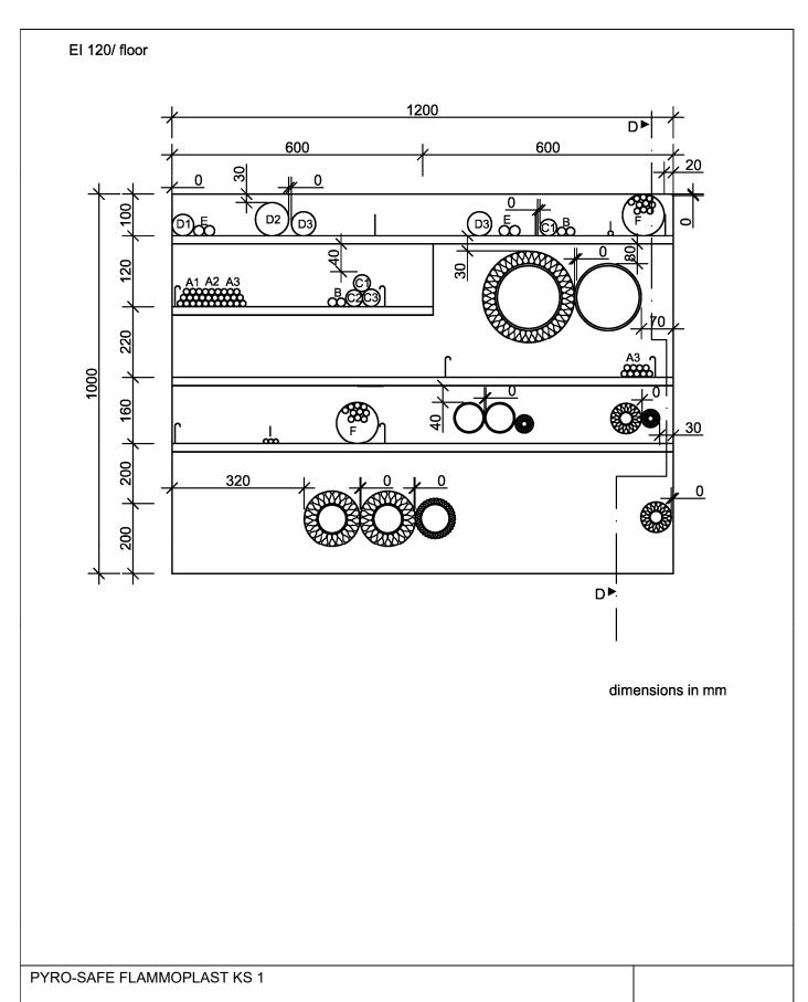
View of the configuration of a penetration seal with the fire resistance class EI 120,
