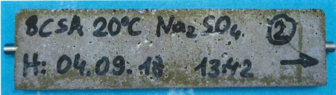
Figure A3.1: Specimens with belitic CSA-Cement "Rapid Set" after 180 days storage \text{Na}_2\text{SO}_4 -solution at 20 °C
