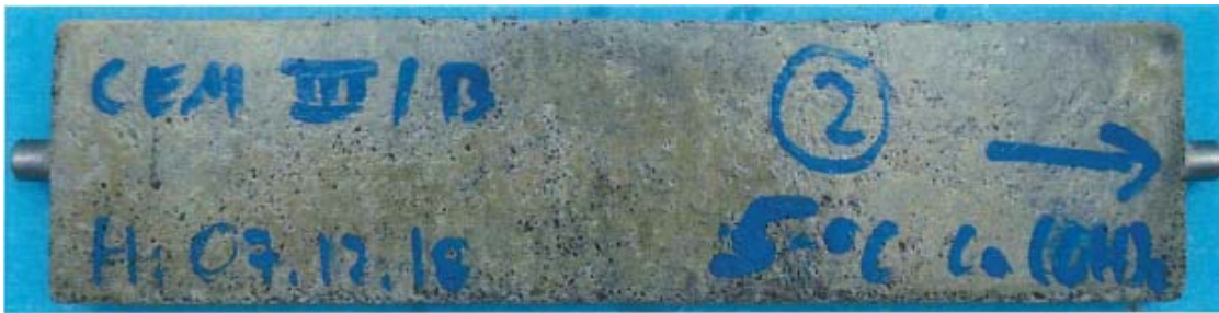
Figure A3.8: Specimens with CEM III/B 42,5 N-SR after 90 days storage in \text{Ca}(\text{OH})_2 -solution at 5 °C
