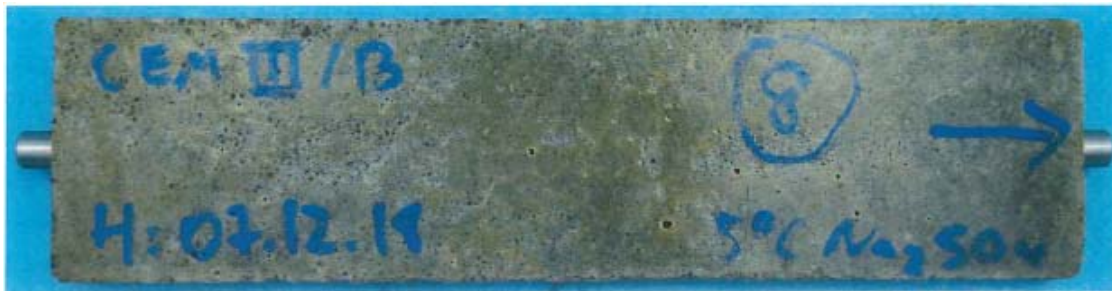
Figure A3.7: Specimens with CEM III/B 42,5 N-SR after 90 days storage in \text{Na}_2\text{SO}_4 -solution at 5 °C
