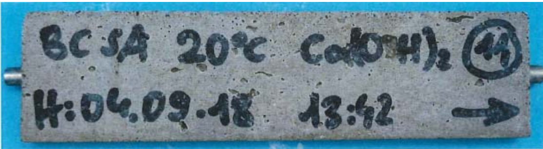
Figure A3.2: Specimens with belitic CSA-Cement "Rapid Set" after 180 days storage in \text{Ca}(\text{OH})_2 -solution at 20 °C
