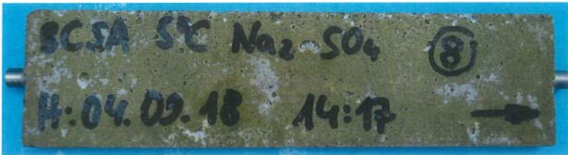
Figure A3.3: Specimens with belitic CSA-Cement "Rapid Set" after 90 days storage in \text{Na}_2\text{SO}_4 -solution at 5 °C
