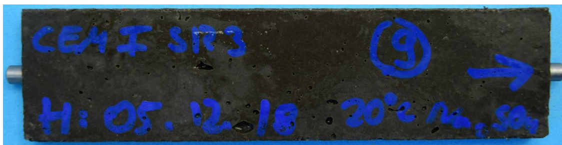
Figure A3.9: Specimens with CEM I 42,5 R-SR3 after 180 days storage \text{Na}_2\text{SO}_4 -solution at 20 °C
