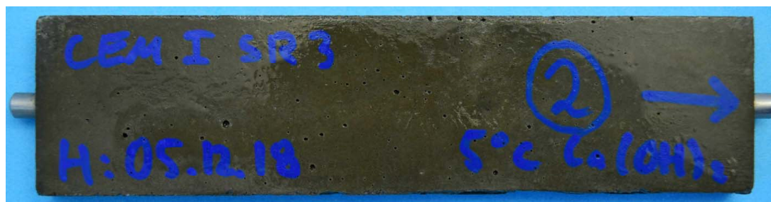
Figure A3.12: Specimens with CEM I 42,5 R-SR3 after 90 days storage in \text{Ca}(\text{OH})_2 -solution at 5 °C
