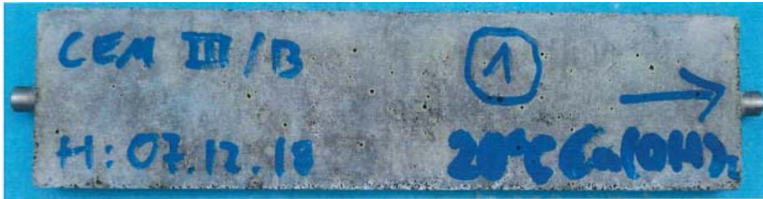
Figure A3.6: Specimens with CEM III/B 42,5 N-SR after 180 days storage in \text{Ca}(\text{OH})_2 -solution at 20 °C
