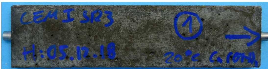
Figure A3.10: Specimens with CEM I 42,5 R-SR3 after 180 days storage in \text{Ca}(\text{OH})_2 -solution at 20 °C
