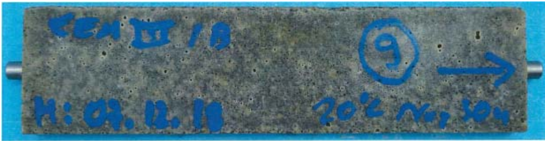
Figure A3.5: Specimens with CEM III/B 42,5 N-SR after 180 days storage \text{Na}_2\text{SO}_4 -solution at 20 °C
