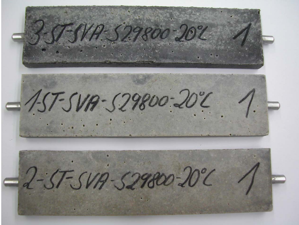
Figure A1: Specimens after 180 days storage in \text{Na}_2\text{O}_4 -solution at 20 °C Top: CEM I; Middle: CEM III/A 52,5 N-SR/LA "Neuwied"; Bottom: CEM III/B
