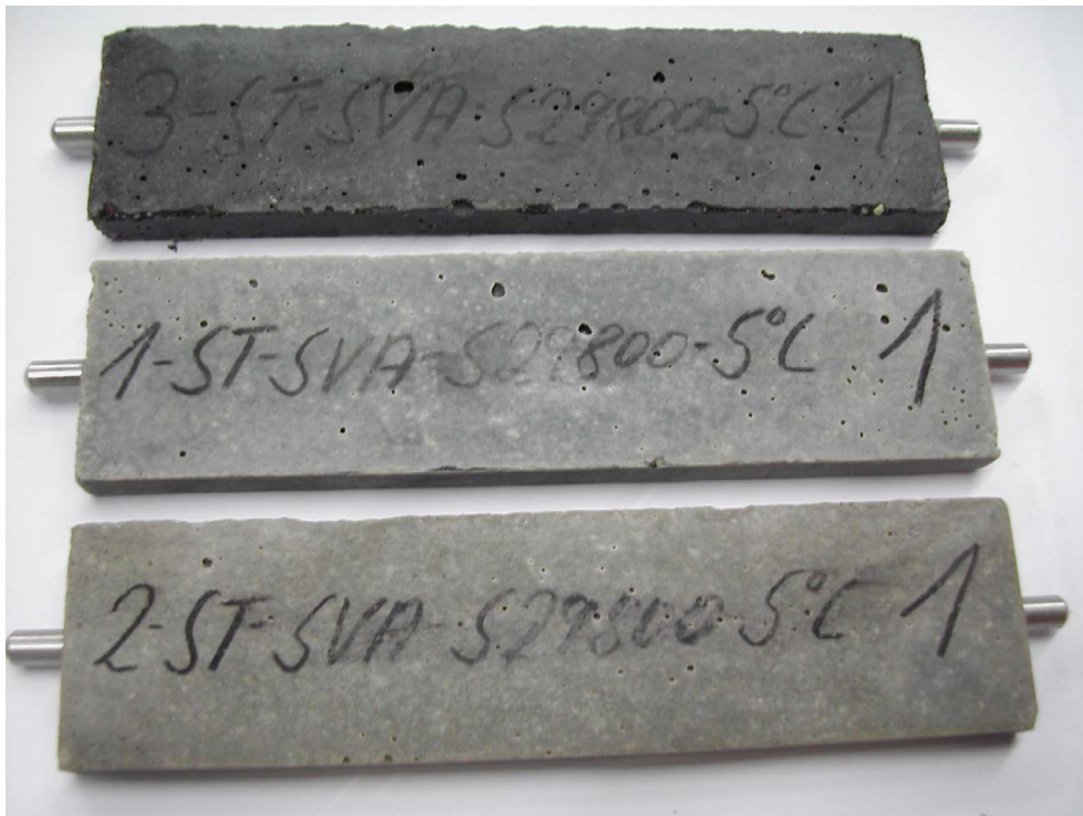
Figure A2: Specimens after 90 days storage in \text{Na}_2\text{O}_4 -solution at 5 °C Top: CEM I; Middle: CEM III/A 52,5 N-SR/LA "Neuwied"; Bottom: CEM III/B
