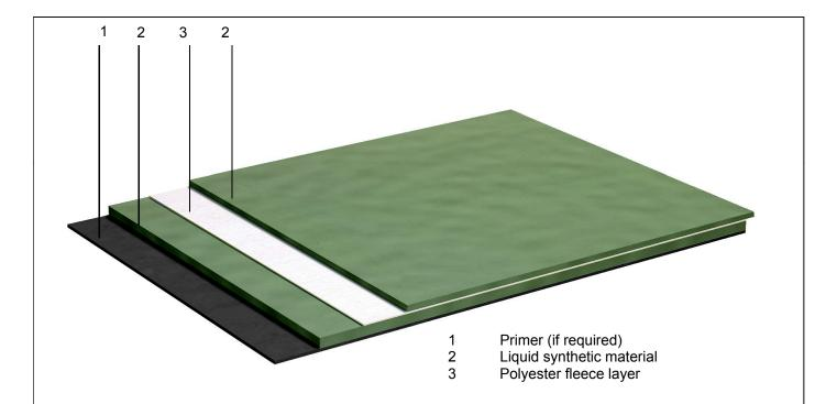
Applicable to the roof waterproofing "BMI SEALOFLEX ENDURA":
