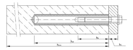
$t_{\text{fix}} \quad = \quad \text{thickness of fixture}$
