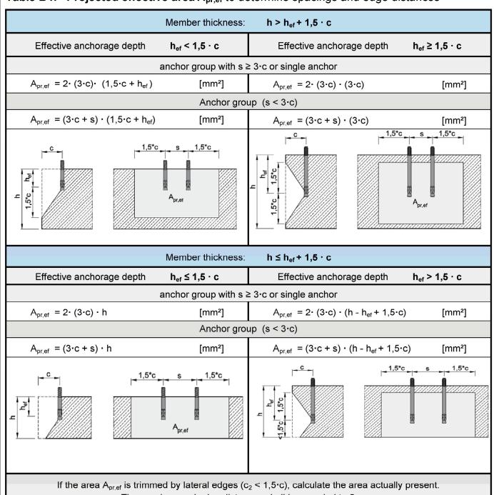
The spacings and edge distances shall be rounded to 5 mm.
