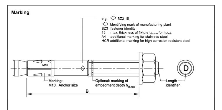
Usable length:  $B = h_{ef} + t_{fix}$
