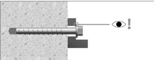
Control of complete setting, full contact of screw head with fixture part.
