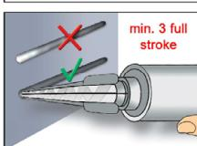
3. Attach the supplied static-mixing nozzle to the cartridge and load the cartridge into the correct dispensing tool. Cut off the foil tube clip before use. For every working interruption longer than the recommended working time (Annex B 6) as well as for new cartridges, a new static-mixer shall be used.
