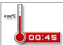
10. Allow the adhesive to cure to the specified time prior to applying any load or torque. Do not move or load the anchor until it is fully cured (attend Annex B 6).
