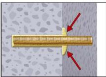
9. Be sure that the anchor is fully seated at the bottom of the hole and that excess mortar is visible at the top of the hole. If these requirements are not maintained, the application has to be renewed. For overhead application the anchor rod shall be fixed (e.g. wedges).
