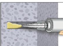
6. Starting from the bottom or back of the cleaned anchor hole, fill the hole up to approximately two-thirds with adhesive. Slowly withdraw the static mixing nozzle as the hole fills to avoid creating air pockets. If the bottom or back of the anchor hole is not reached, an appropriate extension nozzle must be used. Observe the gel-/ working times given in Annex B 6.
