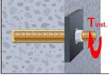
11. After full curing, the add-on part can be installed with up to the max. torque (Table B1 or B3) by using a calibrated torque wrench. It can be optional filled the annular gap between anchor and fixture with mortar. Therefor substitute the washer by the filling washer and connect the mixer reduction nozzle to the tip of the mixer. The annular gap is filled with mortar, when mortar oozes out of the washer.
