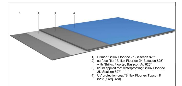
Applicable to the roof waterproofing "Brillux Floortec 2K-Sealcon 827"
