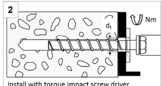
Install with torque impact screw driver or torque wrench
