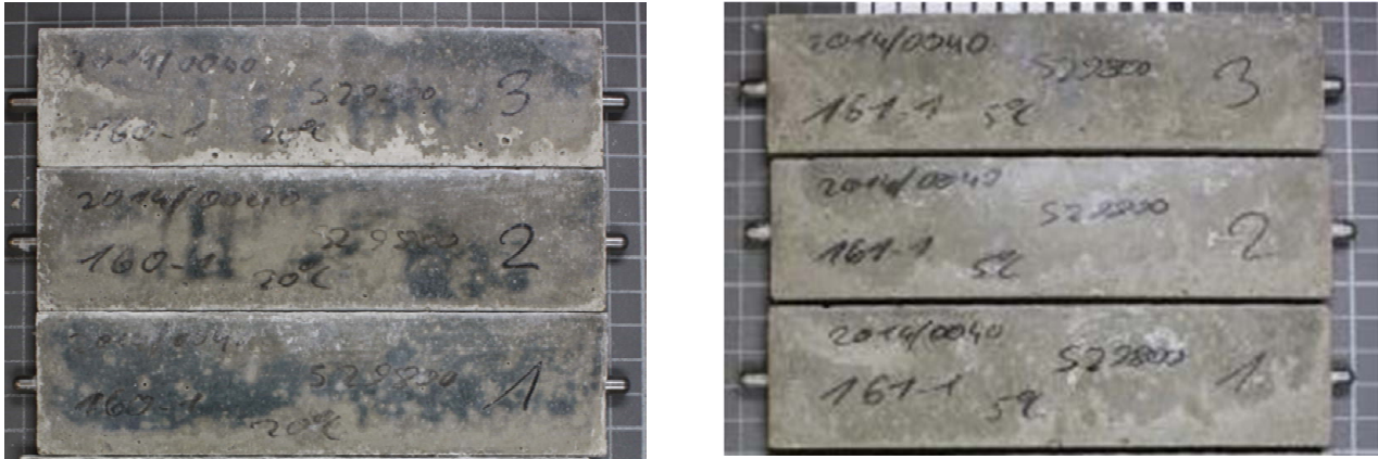
Figure 1: Specimens with CEM III/A 52,5 N-SR "Karlstadt" after sulfate storage; on the left: after 180 days at 20 °C; on the right: after 90 days at 5 °C
