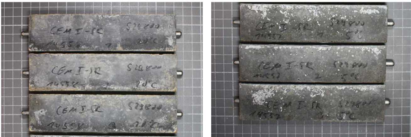
Figure 3: Specimens with CEM I 42,5 N-SR3 after sulfate storage; on the left: after 180 days at 20 °C; on the right: after 90 days at 5 °C
