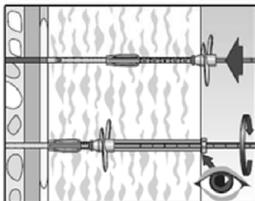
4. Press the anchor with the screw plate tight against the surface of the insulation material, then start screwing-in the anchor.
