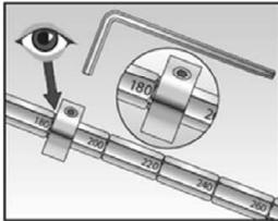
2. Adjust the setting tool ring corresponding to the insulation material thickness  $h_D$  in mm.
