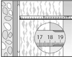
1. Measure insulation thickness  $h_D$
