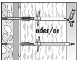
5. The hole in the insulation material must be filled with a suitable foam (illustrated in Annex A1) or must be closed with an appropriate insulation cylinder.
