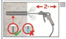
Finally blow the hole clean again with compressed air (min. 6 bar) (Annex B 3) a minimum of two times until return air stream is free of noticeable dust. If the bore hole ground is not reached an extension shall be used.
