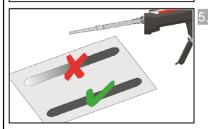
Prior to dispensing into the anchor hole, squeeze out separately a minimum of three full strokes and discard non-uniformly mixed adhesive components until the mortar shows a consistent grey or red colour.
