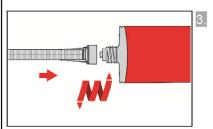
Attach the supplied static-mixing nozzle to the cartridge and load the cartridge into the correct dispensing tool.
