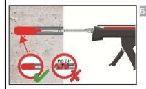
Starting from the bottom or back of the cleaned anchor hole, fill the hole up to approximately two-thirds with adhesive. Slowly withdraw the static mixing nozzle as the hole fills to avoid creating air pockets. If the bottom or back of the anchor hole is not reached, an appropriate extension nozzle must be used. Observe the gel-/ working times given in Table B4.
