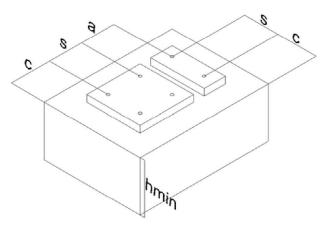
Fixing points with a spacing  $a \le s_{cr,N}$  are considered as a group with a maximum characteristic resistance  $N_{Rk,p}$  acc. to Table 17 – Table 27. For a spacing  $a > s_{cr,N}$  the anchors are considered as single anchors, each with a characteristic resistance  $N_{Rk,p}$  acc. to Table 17 – Table 27.
