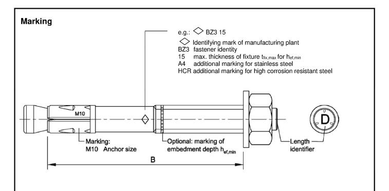
Usable length:  $B = h_{ef} + t_{fix}$
