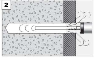
Remove drill dust by vacuuming or blowing of
