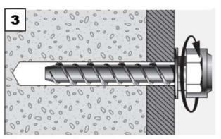
Install with torque impact screw driver or torque wrench
