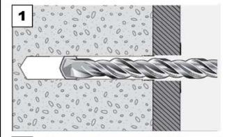
Create hammer drilled or hollow drilled borehole
