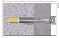
Insert piston plug to back of the hole and inject adhesive. If the bottom or back of the anchor hole is not reached, an appropriate extension nozzle must be used
