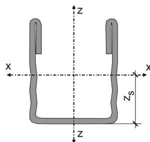
$$\begin{aligned} z_s &= 2,34 \text{ cm} \\ A &= 4,18 \text{ cm}^2 \\ S_x &= 3,50 \text{ cm}^3 \\ I_x &= 14,20 \text{ cm}^4 \\ W_{x,pl} &= 6,99 \text{ cm}^3 \\ W_{x,o} &= 4,80 \text{ cm}^3 \\ W_{x,u} &= 6,08 \text{ cm}^3 \end{aligned}$$
