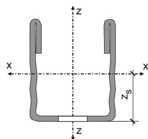
$$\begin{aligned} z_s &= 2,64 \text{ cm} \\ A &= 3,68 \text{ cm}^2 \\ S_x &= 2,90 \text{ cm}^3 \\ I_x &= 11,40 \text{ cm}^4 \\ W_{x,pl} &= 5,80 \text{ cm}^3 \\ W_{x,o} &= 4,30 \text{ cm}^3 \\ W_{x,u} &= 4,33 \text{ cm}^3 \end{aligned}$$
